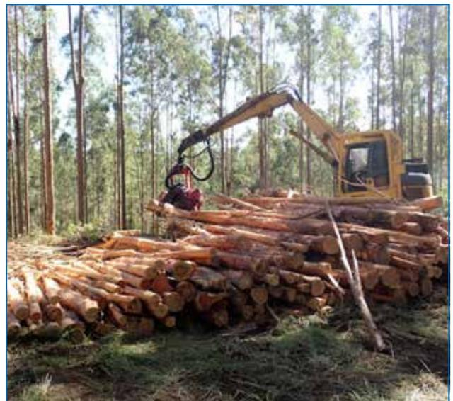
**Figure 10: Initial sorting at log landing**
