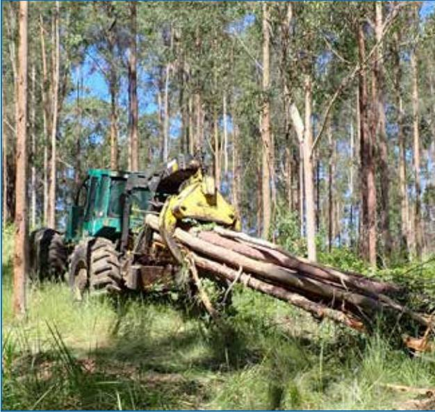
**Figure 7: Skidder removing felled logs to a landing**
